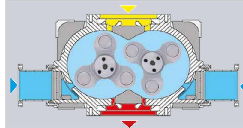
If vacuum (yellow) occurs between the rotor and the casing ambient air (blue) enters the blower block via so-called pre-inlet channels as the rotors continue to turn. The two volume flows subsequently combine and the arising compression heat is dissipated throughout a much larger volume of trapped air. This approach therefore achieves the same discharge temperatures that are produced by normal blower blocks.
