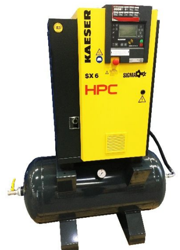
RM (Receiver mount Air Compressor)
